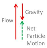
In the vertical, flow is parallel to gravity so particles are continuously re-entrained.
